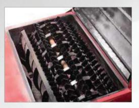
**Twin Tampered Blades**Specially designed blades to cut straw efficiently
