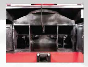
**Double Blower System**Pushes straw efficiently in trolley and removes dust particles
