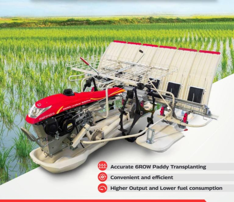
Mahindra Paddy Walker 6ROW is a high accuracy precise Rice Transplanter providing uniform transplanting of paddy seedlings in 6 rows together in the operational field. Its highly reliable gearbox and highly reliable engine ensures lower fuel consumption and higher output in terms of productivity.
