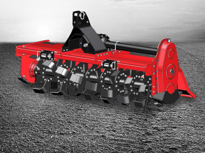
**Mahindra Medium Duty UM Rotavator** is a lightweight series Rotary Tiller specially designed for high performance in medium soils under both dry and wet soil conditions. It is lightweight and robust design makes it a complete solution for progressive farmers tilling needs.
