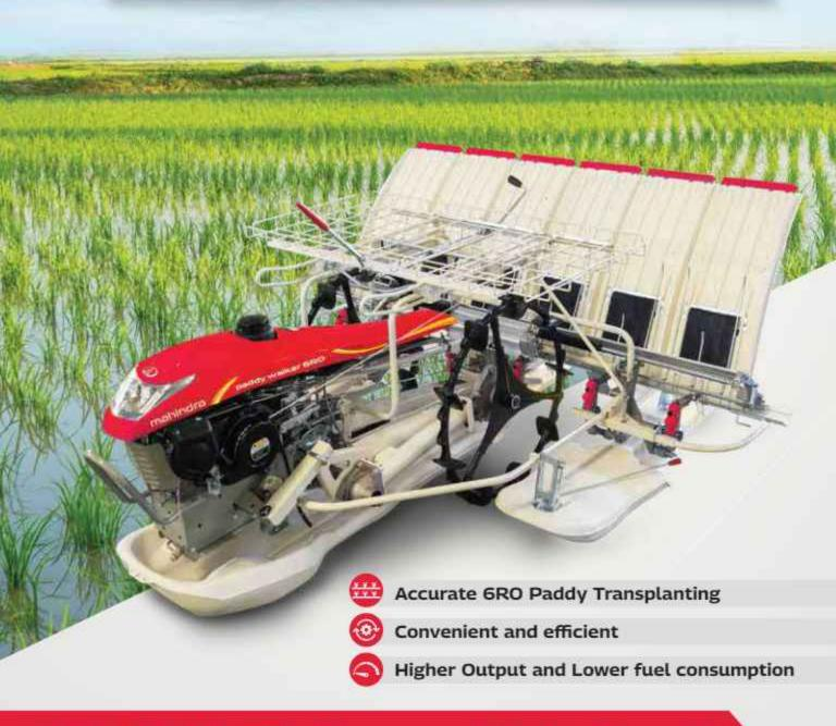
Mahindra Paddy Walker 6RO is a high accuracy precise Rice Transplanter providing uniform transplanting of paddy seedlings in 6 rows together in the operational field. Its highly reliable gearbox and highly reliable engine ensures lower fuel consumption and higher output in terms of productivity.
